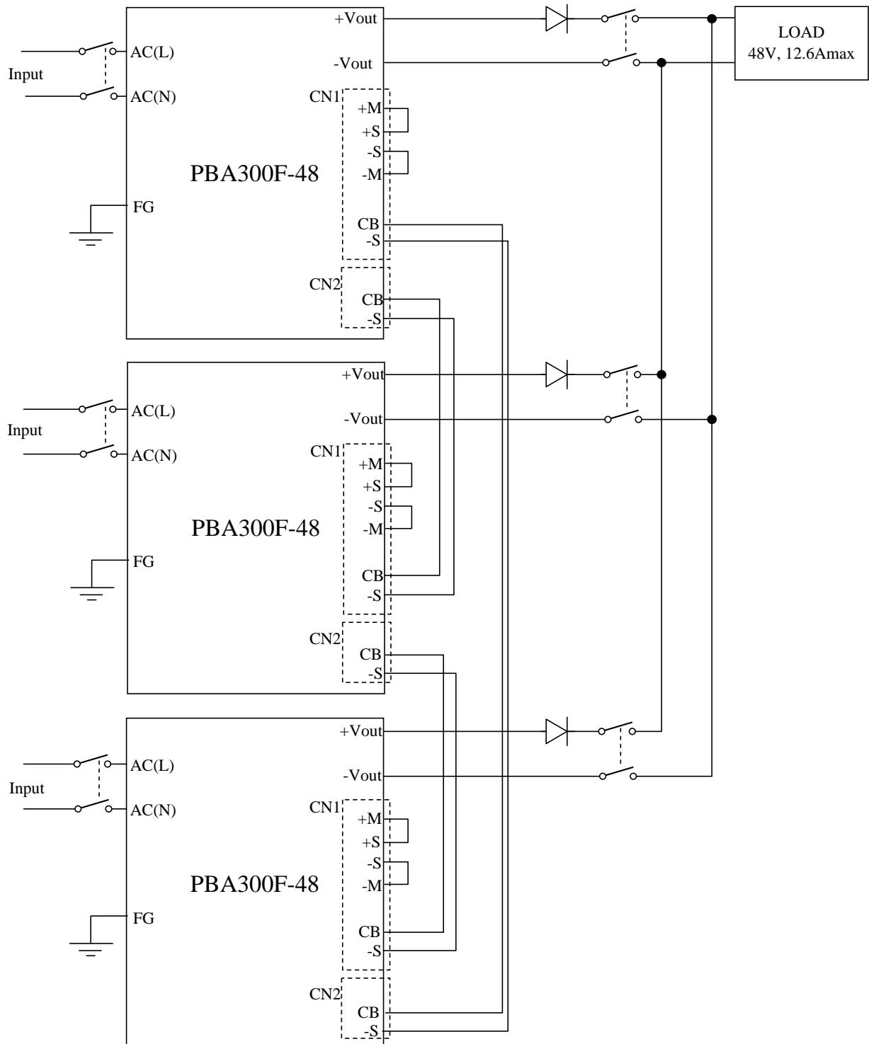
The power supply must be stopped by external switch before it is replaced to the new one.
